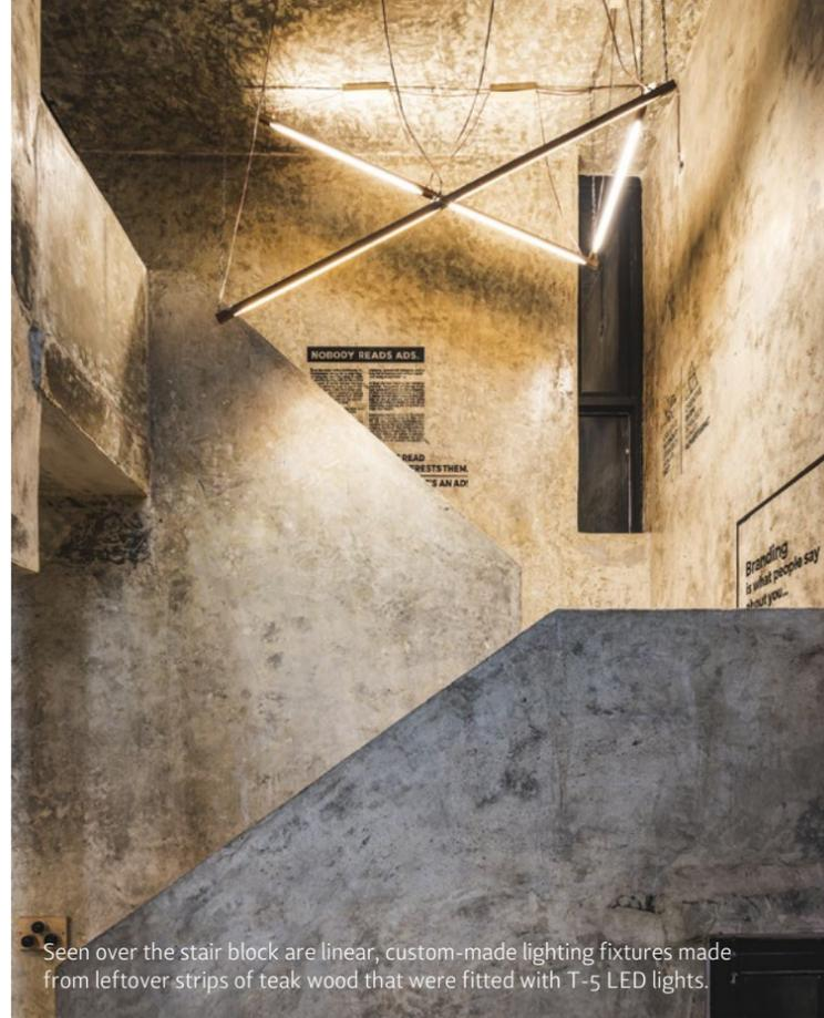
Seen over the stair block are linear, custom-made lighting fixtures made from leftover strips of teak wood that were fitted with T-5 LED lights.
